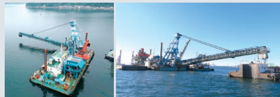
Ocean 3 (Calcia stabilized soil drop mixing vessel)
