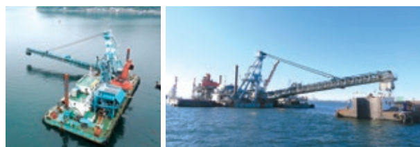
Ocean 3 (Calcia stabilized soil drop mixing vessel)
