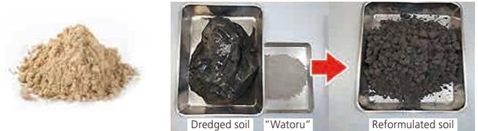
Water-absorbing mud stabilization material "Watoru"
