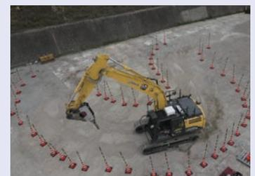
Yard experiment with automatic movement (a backhoe moving automatically, avoiding color cones)
