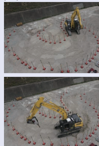
Yard experiment with automatic movement (a backhoe moving automatically, avoiding color cones)
