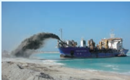
Self-propelling trailing suction hopper dredger, "QUEEN OF PENTA-OCEAN," (currently ANDROMEDA V) put into commission in Singapore (1999)
