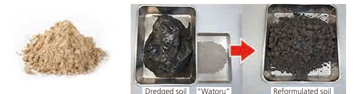
Water-absorbing mud stabilization material “Watoru”
