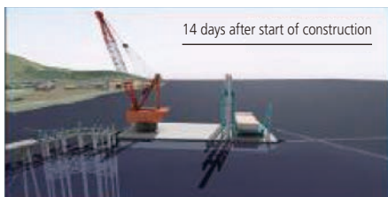
Using a 4D simulation to verify the construction procedures
