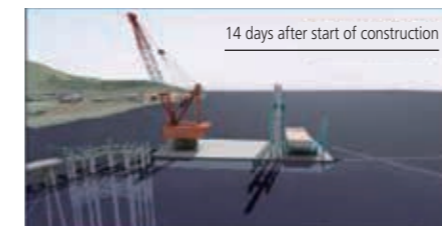
Using a 4D simulation to verify the construction procedures
