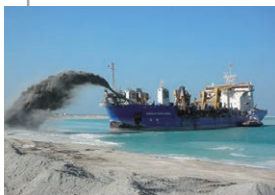
Self-propelling trailing suction hopper dredger, "QUEEN OF PENTA-OCEAN", (currently ANDROMEDA V) put into commission in Singapore (1999)
