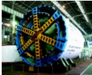
Shield machine worked at Tamagawa project
