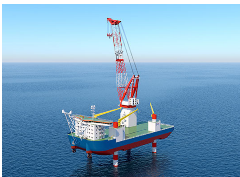
Rendering of the Multipurpose Self-Elevating Platform with a large crane
