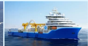
Cable Laying Vessel (CLV)
