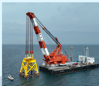
Multi-purpose self-propelling crane vessel CP-5001 (500t lifting capacity)
