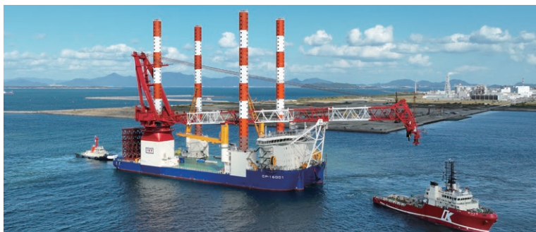
CP-16001: Our second large offshore installation vessel (equipped with a 1,600t lifting capacity crane)
