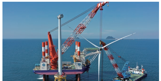
CP-8001: Japan's first offshore installation vessel (equipped with an 800t lifting capacity crane)
