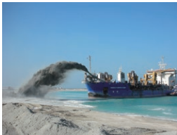
Self-propelling trailing suction hopper dredger, "QUEEN OF PENTA-OCEAN," (currently ANDROMEDA V) put into commission in Singapore (1999)
