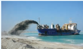
Self-propelling trailing suction hopper dredger, "QUEEN OF PENTA-OCEAN," (currently ANDROMEDA V) put into commission in Singapore (1999)
