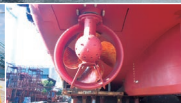
Propulsion engine that can swivel in any direction
