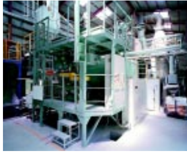
Incinerator ash-granulating/sintering system
