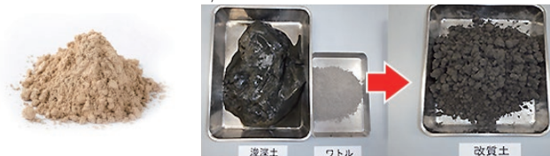
Water-absorbing mud stabilization material "Watoru"
