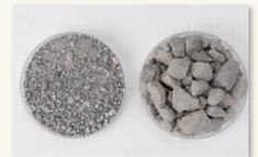
Recycled fine aggregates (left) and recycled coarse aggregates (right)
