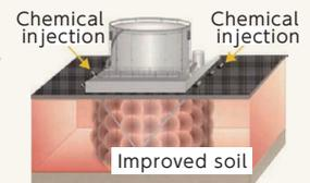
Mechanism of Infiltration Solidification Processing Method
