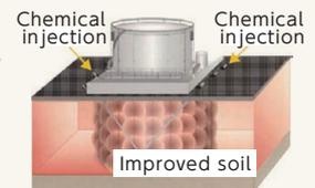
Mechanism of Infiltration Solidification Processing Method
