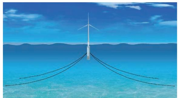
Conceptual image of a spar-type floating structured offshore wind power
