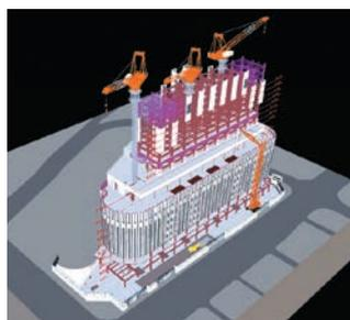
Examination of construction procedures by BIM
